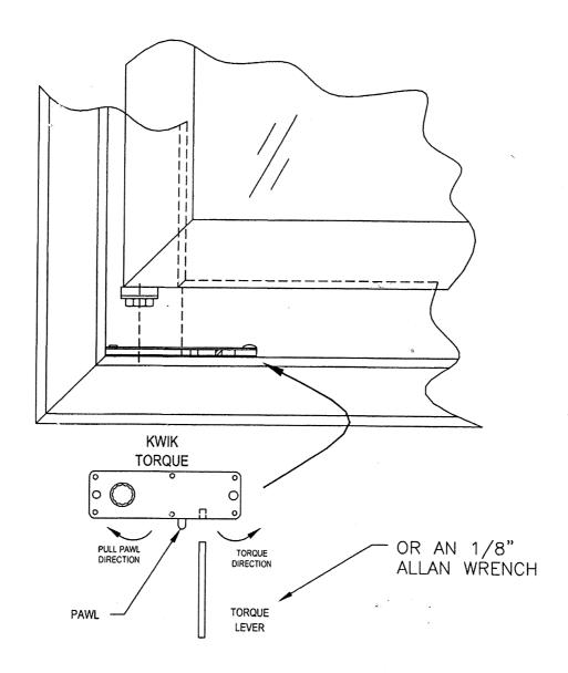
WITH DOOR IN CLOSED POSITION, YOU WILL ENGAGE THE TORQUE OPERATED SELF CLOSING MECHANISM:
